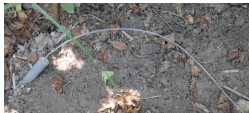
Figure 7.12. Syringes were removed from macrorhizons by chewing through the connecting tube (top). A macrorhizon where the connecting tube was pulled out and eventually the syringe removed (bottom)
