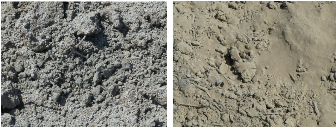
Figure 6.10. Comparison of the Norwegian (left) and Grecian Magnesite (right) treatments after manual application of 4\text{kg}/\text{m}^2 on the experimental plots. Note the granular texture of the Norwegian rock dust, resulting from its moisture content, as opposed to the blanket of powder of the Grecian Magnesite material, representative also of the application of the 4 other rock dusts.
