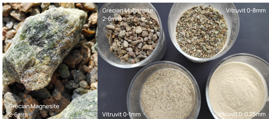
Figure 4.2. Photographs of larger rock pieces and 2-6 mm olivine rich "dunite" provided by Grecian Magnesite, as well as the three grainsize fractions of "olivine" provided by Vitruvit, in the autumn of 2020.
