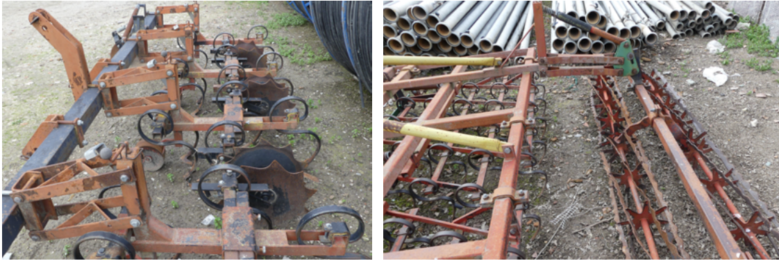
Figure 6.31. The two final tools pulled behind the tractor to prepare the soil for sowing by breaking up and 'raking' through the top soil layer.
