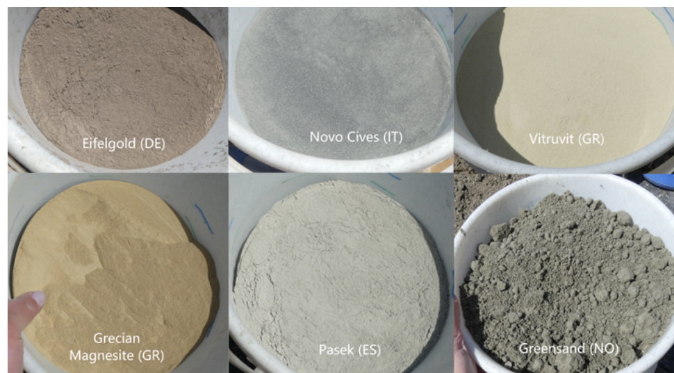
Figure 4.3. Photographs of the 6 different rock dusts applied on the cotton field, identified by the name of the company we obtained them from and the country code of their origin. Notice the clotting in the partially wet Norwegian rock dust on the bottom right.
