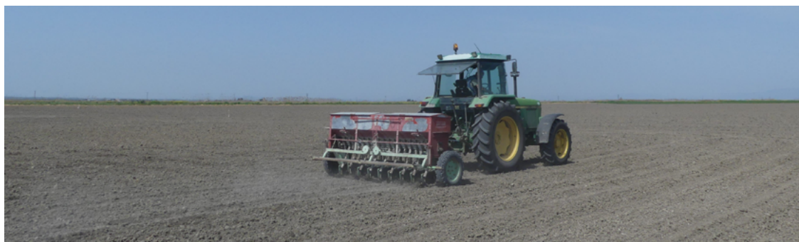
Figure 6.27. Despite many rounds across the pilot – which result in the bad effect of soil compaction – the biochar is barely falling from the wheat-sowing machine. Another piece of equipment is needed for mechanical application of the biochar.
