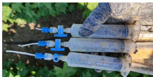
Figure 7.11. Intense sunlight made the plastic of this syringe so brittle that the connection tip (left) broke off, as well as part of the back to secure the vacuum (right). Such syringes were replaced with new ones.
