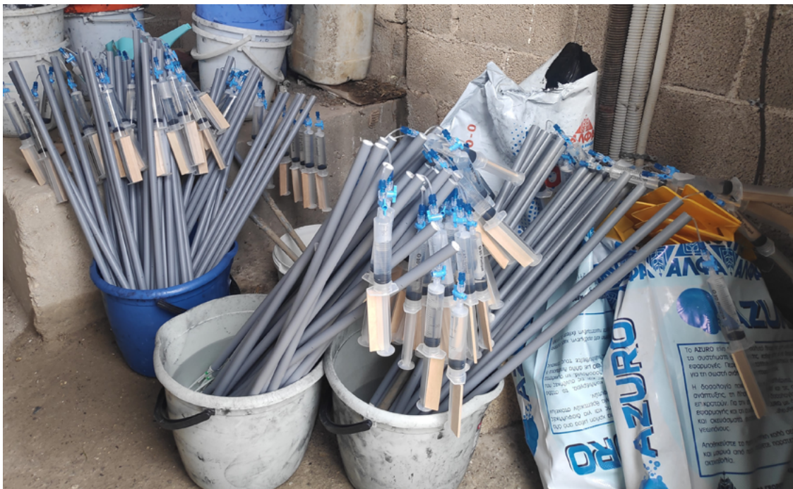
Figure 6.40. Macrorhizons prepared for installation. Notice that most of the syringes are at least half-full of water.
