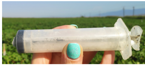
Figure 7.11. Intense sunlight made the plastic of this syringe so brittle that the connection tip (left) broke off, as well as part of the back to secure the vacuum (right). Such syringes were replaced with new ones.
