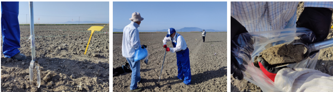
Figure 7.3. The upper 30 cm of soil are sampled with an auger, collecting multiple small cores across a plot which are combined into a single composite soil sample.
