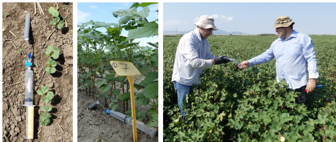
Figure 7.5. Growth of the cotton plants as observed during macrorhizon water sampling on 13 May (left), 11 June (middle) and 19 August (right). The average final height of the cotton plants is about 1 meter. Notice how in the first ca. 1.5 month the plastic syringes are exposed to full, direct sunlight before getting any shadow from the growing cotton plants.
