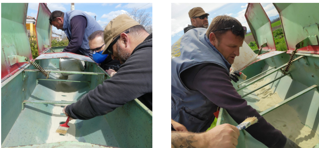
Figure 6.12. Initial testing of the wheat-sowing machine for mechanical rock dust application. Left adding weighed buckets of rock dust to the seed container and evenly spreading it out. Right for homogenous application of the rock dust to the field, it is important that all 18 seeding feeders continuously receive rock dust through the top openings.
