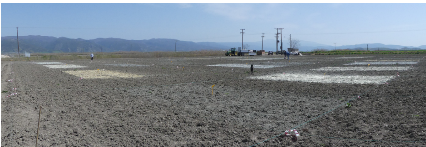
Figure 6.11. Overview of the experimental area after manual application of the six olivine rich rock dusts
