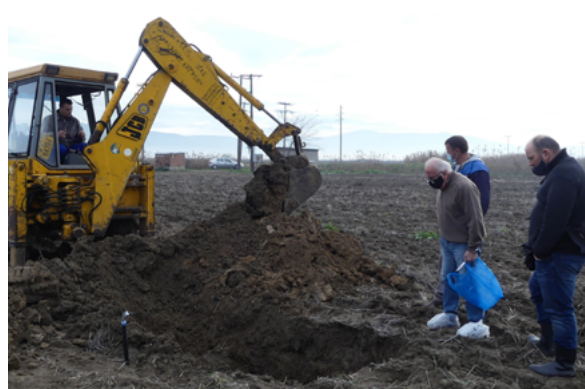
Figure 3.7. JCB digger opening up a full soil profile for more detailed soil characterization and sampling.
