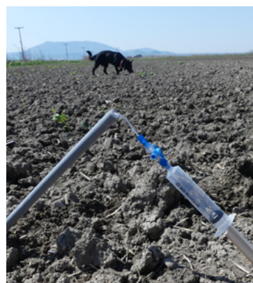
Figure 6.43. Macrorhizon installed in the field with vacuum maintained by inserting the wooden retainer into the syringe.
