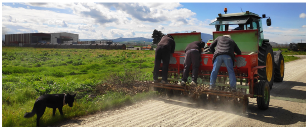
Figure 6.13. Testing and calibrating the wheat sowing machine for mechanical rock dust application on the pilot plots.
