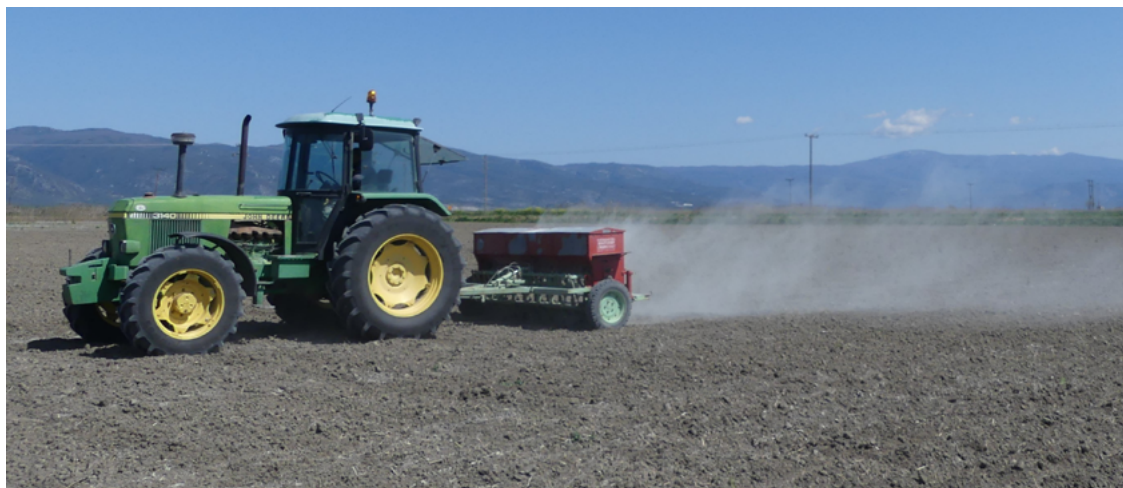
Figure 6.16. At the start of a mechanical rock dust application round, the weight of the rock dust itself is sufficient for continuous spreading down the seed feeders. The field already has application traces, indicating this is the second and last round.
