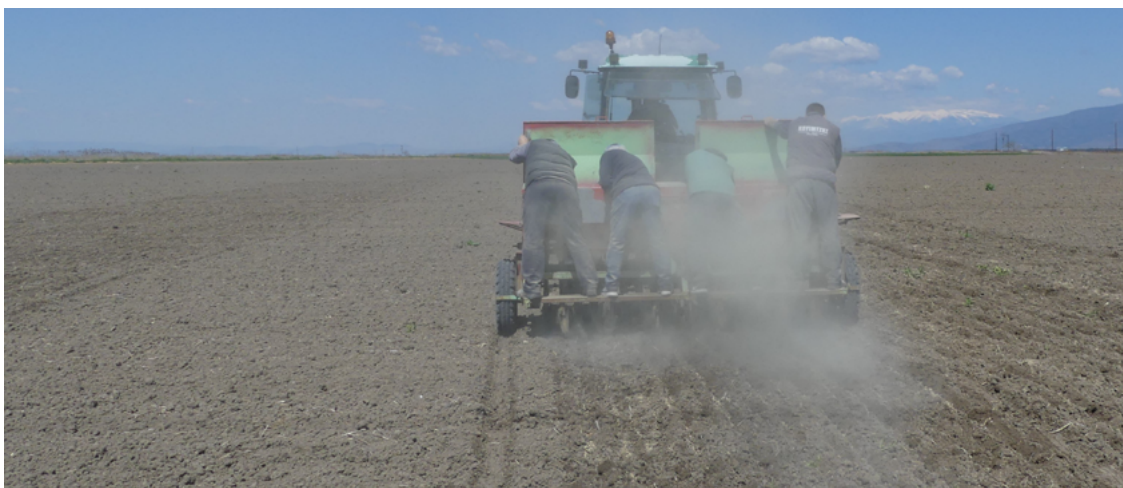
Figure 6.17. Towards the end of a round, four people on the back of the wheat-sowing machine push the remaining rock dust towards the sowing feeders to assure continuous application. Note the traces in the centre and the left part of the photo: this is the end of a first application round; each round is done by driving concentrically inward of the pilot plot.
