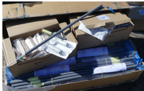
Figure 6.38. The macrorhizons and syringes to create vacuum.
