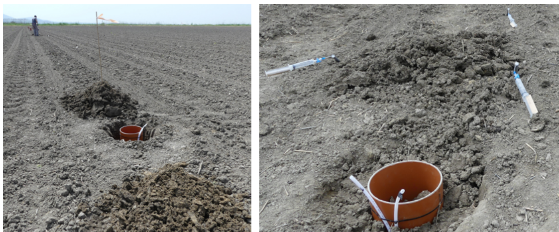
Figure 6.46. Left: Lysimeter placed inside a hole dug in the pilot area – note the separation of the soil horizons in the two distinct heaps in front of and behind the lysimeter. Right: Lysimeter partially filled up and worked back into the soil in one of the experimental plots. The 5 macrorhizons above it are sampling water from the top area of the picture, the lysimeter placement will not interfere with the soil system where they sample water from.
